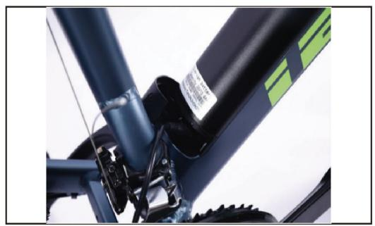
Battery charging method 2:Turn the key in an anticlockwise direction to take out the battery set.
