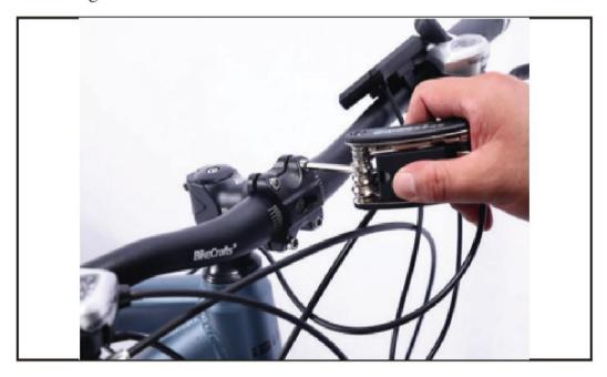
Step 4: Inserting the handle bar into the connector, screw up four screws and adjusting again then tighten all screws.
