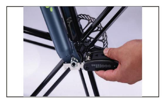
Step 2: Installing front tire on the front fork and then screw up.
