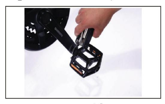
Step 7: Installing pedal with label "R" on right side clockwise, "L" on left side anticlockwise. Must tighten them at the first time.
