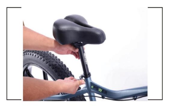
Step 6: Inserting the seat post into the seat post clamp, adjusting height and then locking the buckle.
